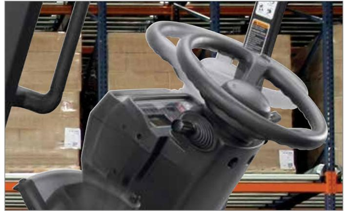
**Hydraulic Levers** – These are ergonomically-designed to fit the operator's hand and posture, while providing the accuracy needed for precise maneuvering.
