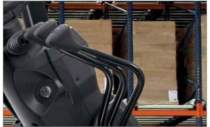
**Optional Fingertip Controls** – These controls are mounted to the armrest and allow the operator to easily manipulate the hydraulic system from a comfortable position.
