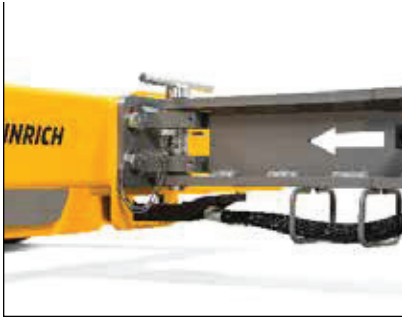
Electrical connection for trailers (GTE 312)
