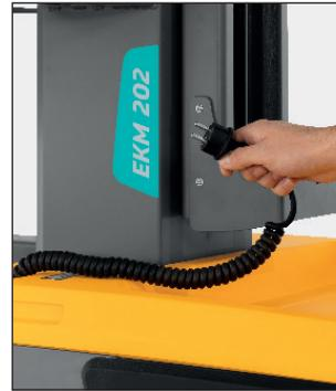
On-board charger with integrated spiral cable
