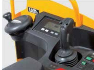
All drive and lift functions are controlled by the multifunction joystick.
