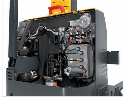
Sealed AC motor, controllers and connectors
