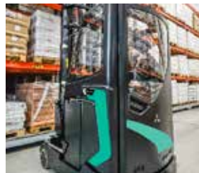
Cold storage cabin
