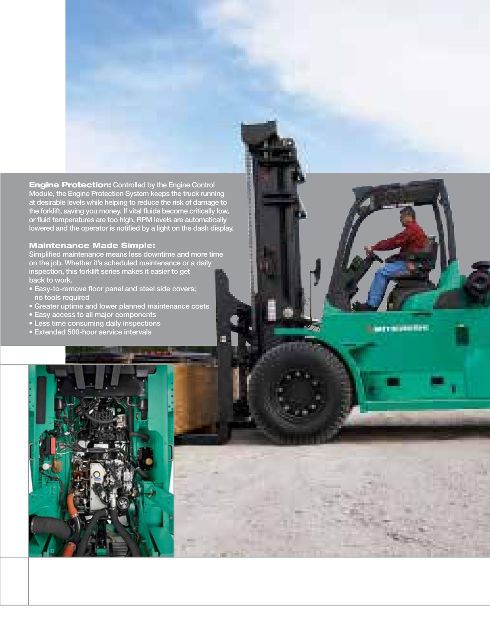
**Engine Protection:** Controlled by the Engine Control Module, the Engine Protection System keeps the truck running at desirable levels while helping to reduce the risk of damage to the forklift, saving you money. If vital fluids become critically low, or fluid temperatures are too high, RPM levels are automatically lowered and the operator is notified by a light on the dash display.
