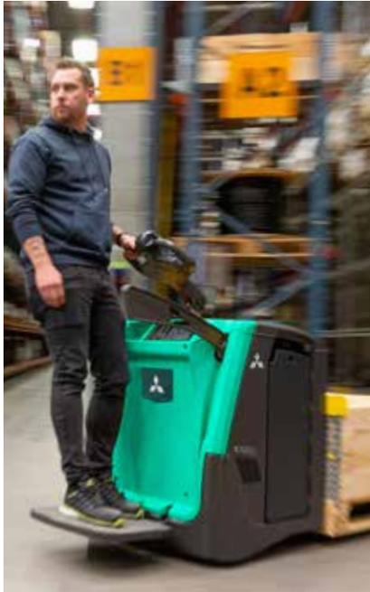
The patented DriveSteady system ensures outstanding drive wheel pressures, excellent shock absorption and side stability when cornering - making PREMIA EM a milestone power pallet truck.
