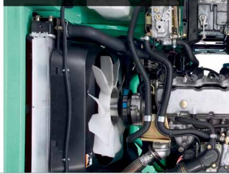
**Cool And Quiet:** The forklift's fan and radiator system is equipped with a horizontal cross flow cooling system to help keep the engine cool and functioning at peak performance. The corrugated design provides optimal heat exchange, while the aluminum core helps to prevent corrosion. The direct drive fan also reduces noise and necessary maintenance, benefiting your operators and your business.
