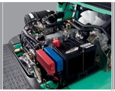
Easy Service Access: Tool-free access to the engine compartment makes routine maintenance, such as cleaning radiator fins, much easier. Additionally, the Vehicle Control Module is conveniently located under the dashboard cup holder, making it readily accessible.
