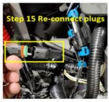
Plug the access control plug back together and verify the truck now has travel.
