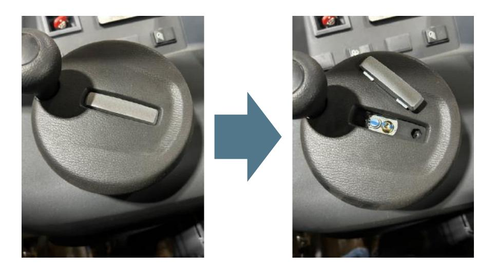
**Step 4:** Remove the snap ring and cap screw, remove the tiller, then remove the upper dash cover.
