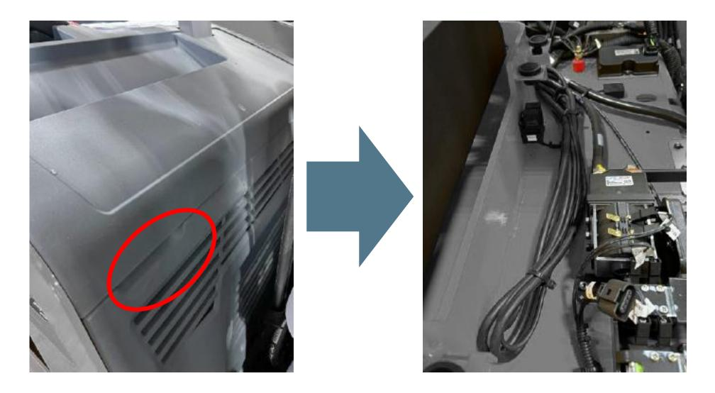
**Step 3:** Pop the plastic insert out of the steering tiller using a small screwdriver.
