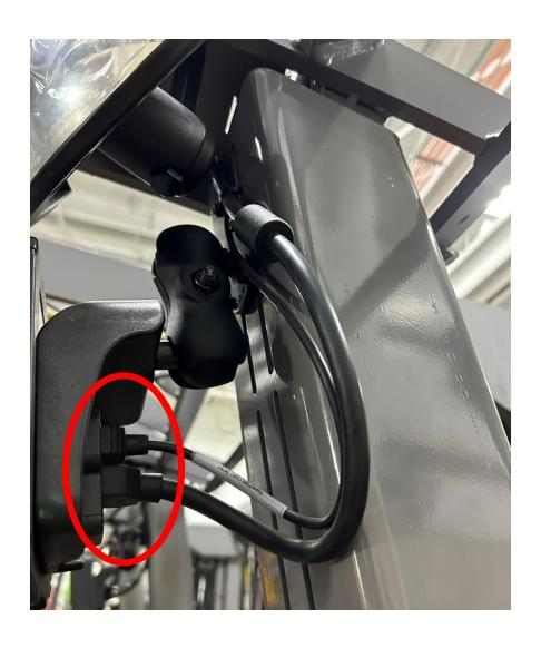
**Step 13:** Connect the battery and power on the truck to verify the VAC unit is powered.
