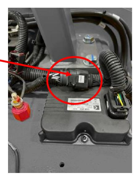
**Step 6:** Install the impact sensor to the frame as in the indicated picture/drawing.
