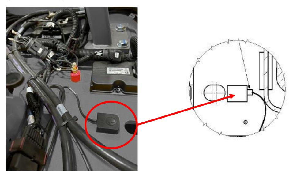
Step 7: Remove the OHG option bracket by removing the screws on the back.
