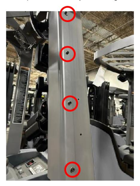
**Step 8:** Install the RAM mount to the OHG option bracket, then re-install the OHG option bracket.
