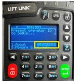
1. Press 2 on the keypad to select "Config" and then press the green ENTER button.
