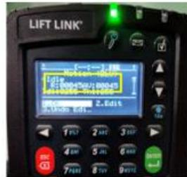
9. Press the throttle in the  fwd  or rev travel direction. Verify that the **R & AV** numerical values change. Perform this step for both  fwd  & rev throttle. Confirm **R & AV** values change press Red ESC button.
