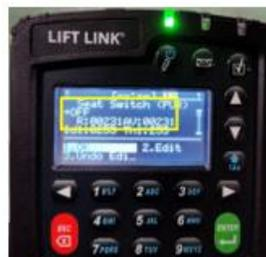
13. Depress the seat or step on the operator presence switch & verify the **R & AV** numerical numbers change. Confirm the **R&AV** number change & press the Red ESC button several times to return to the main start screen. You should see a key or wrench symbol.
