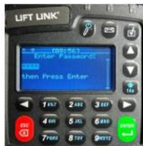
3. Use the keypad to enter **2378** and then press the green ENTER button. (Note: truck able to run once this step is complete).
