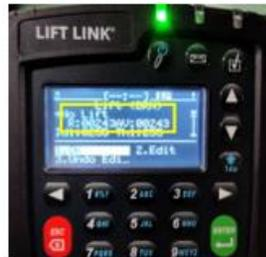
11. Press the up button and verify that the **R & AV** numerical numbers change. Confirm the R & AV numbers change & then press the Red ESC button.
