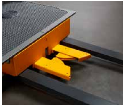
Simplified pallet retention on the EKS 414s
