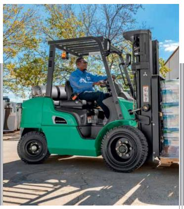
**SmoothShift**: Provides smooth direction shift changes, resulting in reduced transmission shift shock, protecting the Drivetrain from full-speed shifts in direction, plus reduced tire spin, for increased tire life. This system helps reduce possible damage to the Driveline components due to the shock of high speed shifts, while also reducing tire spin to extend tire life. For LP/LPG models only.
