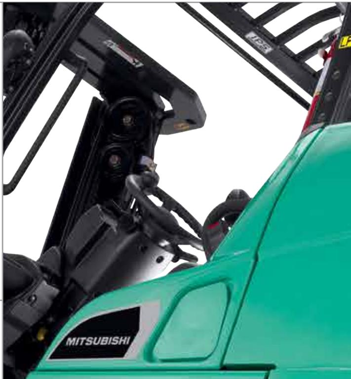
Ground speed control allows you to set limits for the forklift's top speeds, especially useful in applications with pedestrian traffic.
