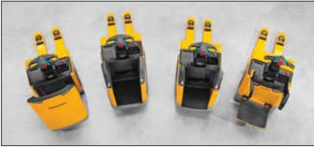
With four different stand-on platforms, users can also set the height of the platform and the level of comfort to suit their specific requirements.
