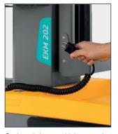
On-board charger with integrated spiral cable
