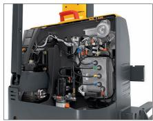
Sealed AC motor, controllers and connectors
