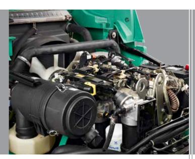
Engine Protection: Regulated by the Vehicle Control Module, the Engine Protection System keeps the truck running at desirable levels while helping to prevent damage to the forklift, saving you money. If the vital fluids become critically low, RPM levels are automatically lowered and the operator is immediately notified by a light on the dash display.
