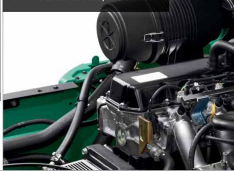
Cool And Quiet: The forklift's fan and radiator system is equipped with a horizontal cross flow cooling system to help keep the engine cool and functioning at peak performance. The corrugated design provides optimal heat exchange, while the aluminum core helps to prevent corrosion. The direct drive fan also reduces noise and necessary maintenance, benefiting your operators and your business.
